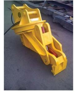
Max. Hyd. Pressure 210 Bar Min. Hyd. Pressure 90 Bar Rotator Max Hyd. press. 150 Bar Body Colour 08E51 Yellow Jaw and cylinder Signal Red
